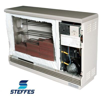
During Off-Peak hours, the ETS unit's heating elements convert electricity to heat which is stored in high-density ceramic bricks. The bricks are surrounded by high-efficiency insulation which allows them to hold great amounts of heat for long periods of time. A fan evenly and quietly distributes the heat to your home during higher cost, On-Peak hours and built-in thermostats allow you to easily maintain a desired temperature.
