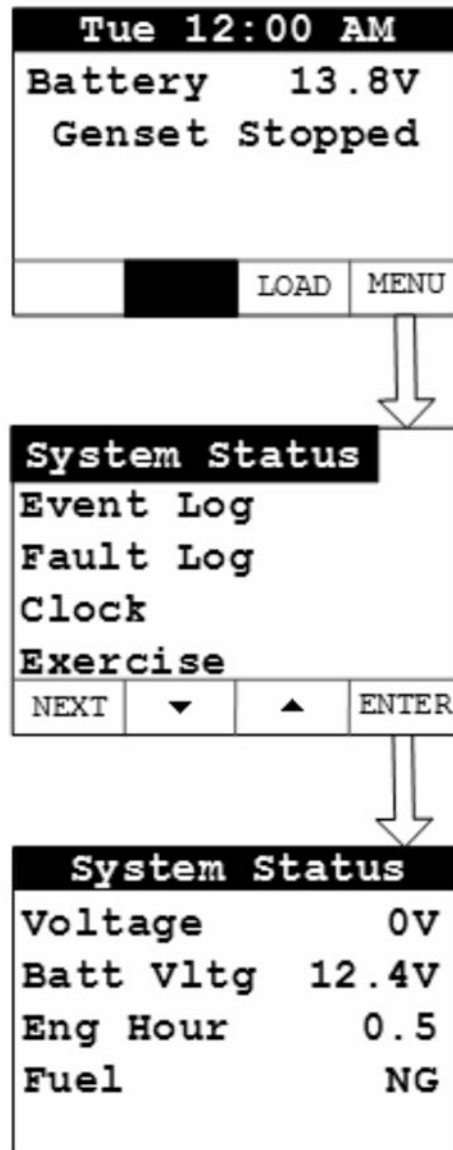
FIGURE 14. SYSTEM STATUS SCREEN
