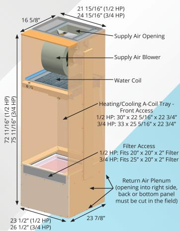
The Steffes Air Handler includes a return plenum, supply air blower, water coil, and air filter. The air handler's variable speed blower incorporates an ECM motor that automatically adjusts its speed to achieve the appropriate CFM for the thermostat input received.
